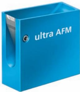
The high quality Diatome diamond knives are not just perfect for producing ultra-thin and semi-thin sections, but also for surfacing sectioning of all kinds of biological and industrial specimens for AFM investigation.
